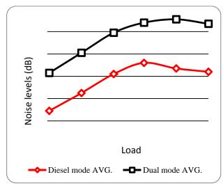
Fig. 4 Variation of noise levels with variation in load.
