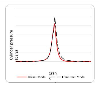
Fig. 1 Variation of cylinder pressure with crank angle.
