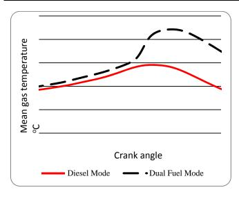
Fig. 2: Variations of mean gas temperature with crank angle.
